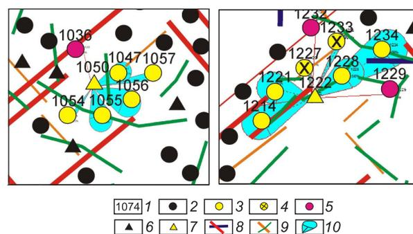
**Fig. 11.** Migration of the tracer fluid from injectors to producers: test results (Urna field).
